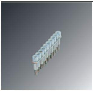
Fixed bridge, for cross connections in the terminal center, with fixed crimped rolls, screw heads with insulating collar as shock protection, 10-pos., divisible
